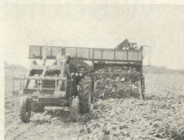
New Pickle Harvester with bulk bin 2000 lb. capacity. Can harvest 1 acre per hour.
