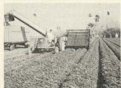
Parsley cutter and loader. Capacity 1 ton per minute. Also harvests Spinach, turnip greens, collards and kale. Also beet greens and mustard greens.
